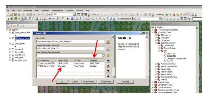
w. Contour lines can be made from the new TIN layer, Open ArcToolbox, go to 3D Analysis Tools > Terrain and TIN Surface > Surface Contour
