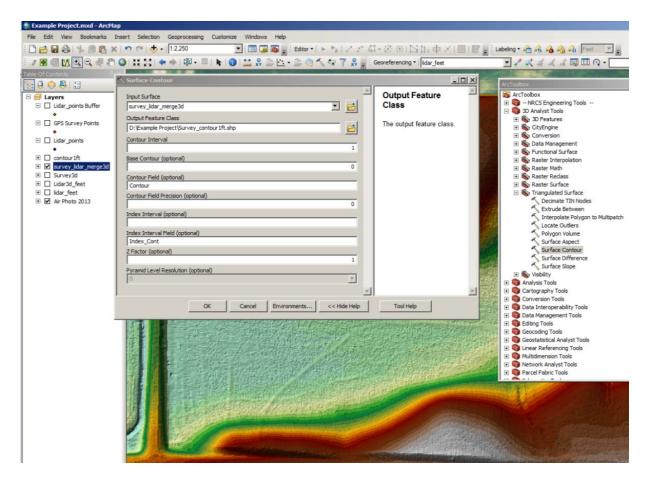
x. This merged TIN layer can be supplemented and used in the dike building tutorial instead of pure LIDAR data. In the dike building exercise you need a TIN in Meters units so add a step of creating a new field in the attribute table for both the lidar points layer as well as the survey points layer and do a conversion calculation to meters. Then continue with the rest of the steps to create the TIN with the **meters** as the **height** and **tag** value field.
