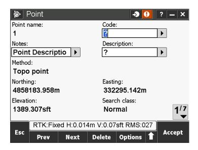
9. Finishing Survey – Hit the Escape key until it asks to stop the survey and you say yes to the option to power down receiver. If you are finished with field work power off the controller by holding down the green power key until the power menu screen comes up which you choose shut down.
