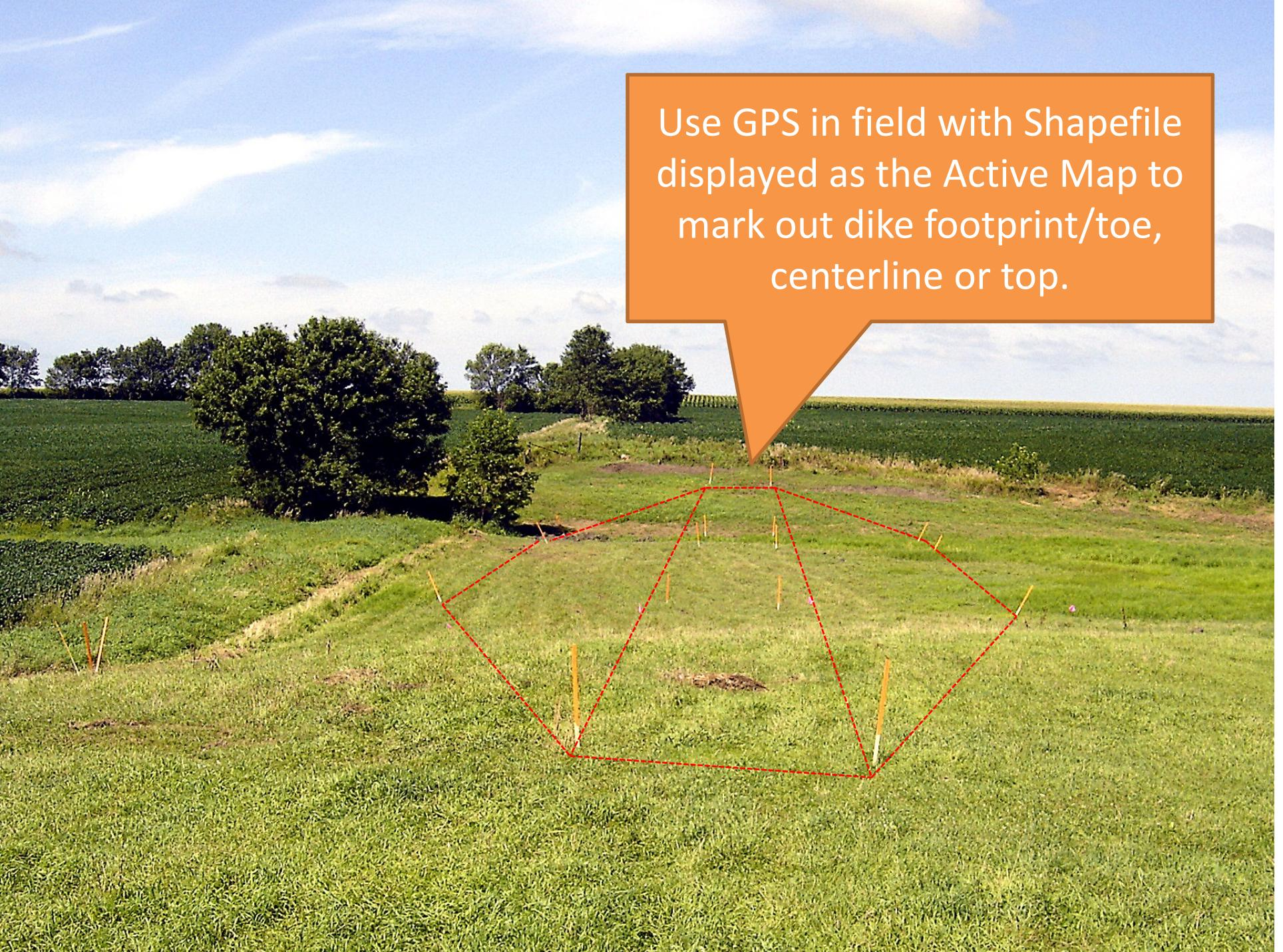
Use GPS in field with Shapefile displayed as the Active Map to mark out dike footprint/toe, centerline or top.
